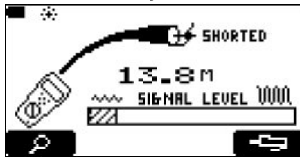
the middle of a cable. Figure 2. Measure length, verify continuity, and measure the distance to shorts and breaks.
