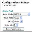
Step 2. Select the print mode, baud rate, parity, and data bits from the pull-down lists.
