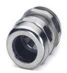
Cable gland, cable gland material: Nickel-plated brass, external cable diameter 11 mm  $\dots$  16 mm, shielding: yes, connecting thread: M25 x 1.5, color: silver, with O-ring
