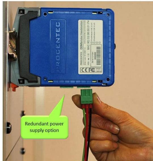
Powering the Head Station
