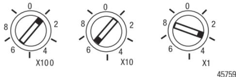
When the switches are set to a valid number, the I/O block's IP address is 192.168.1.xxx (where xxx represents the number set on the switches). The I/O block's subnet mask is 255.255.255.0 and the gateway address is set to 0.0.0.0. When the I/O block uses the network address set on the switches, the I/O block does not have a host name assigned to it or use any Domain Name Server.
