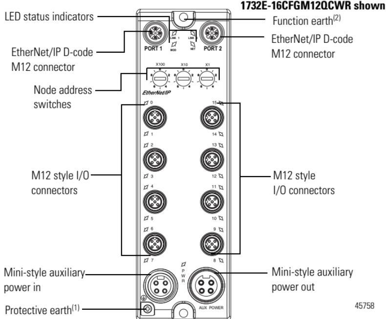
(1) Protective Earth is provided for the grounding of field devices and is internally connected to each Pin 5 of the M12 I/O connectors. See I/O Connectors on page 9.
