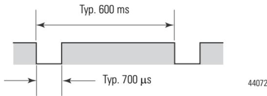
While safety outputs are in an on state, the signal sequence shown in the figure is output continuously for fault diagnosis when output pulse testing is enabled. Confirm response time of device connected to safety outputs so the device does not malfunction due to off pulse.
