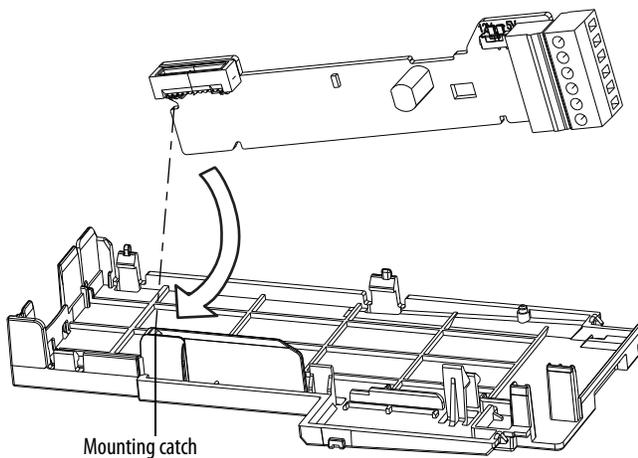
Note: Incremental Encoder Input is for PowerFlex 525 only. You can install both the communication adapter and optional Incremental Encoder Input on the same Control Module Back Cover.
